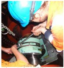
Above: Qualtex staff lifting bearing into 8.5 mw motor
